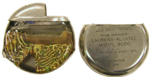
Figure 2.2. A plutonium powered pacemaker. The plutonium has been removed; it fit into the slot on the top left. Hundreds of these were implanted in patients with no ill effects. Cold fusion will also scale down to devices this size or smaller, and it will scale up to any size you like. http://www.orau.org/ptp/collection/Miscellaneous/pacemaker.htm
