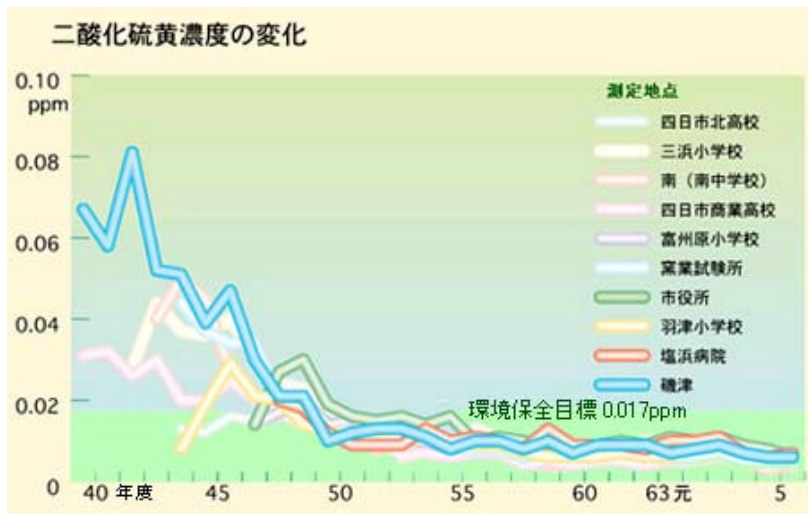
Figure 16.2. The sulfur dioxide concentration levels at Yokkaichi from the 1960s to the present, measured at various locations in the city. The environmental target is 0.017 ppm, shown in the green bar at the bottom of the graph. The peak was in 1967 (Showa 42).
